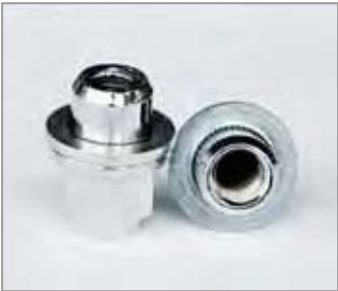
Accepts only TOYOTA O.E. flat seat wheel nuts
