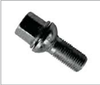
Accepts only VOLKSWAGEN O.E. ball seat wheel bolts
